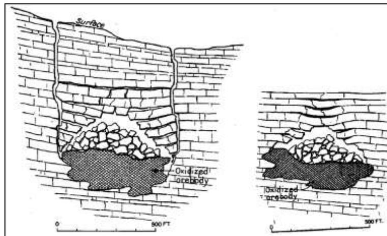
Figure 3 Subsidence features in thin-bedded limestone, near surface (left) and at depth (right) (Wisser, 1927, Figs. 7, 8)
