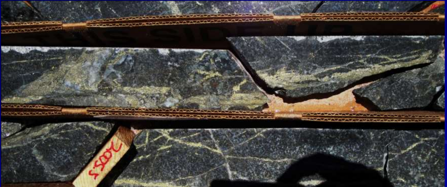
High grade copper ore as chalcopyrite-quartz-phlogopite veins hosted in biotitized diabase In core from Resolution Cu-Mo-Ag deposit. Photo by S. Keith early June, 2010.
